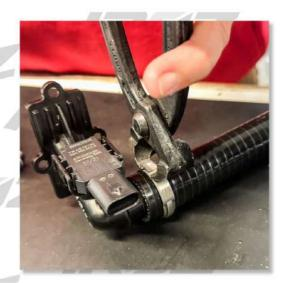
Slip on the upgraded IMS Turbo Inlet Breather Adapter hose onto the sensor you just cut.
